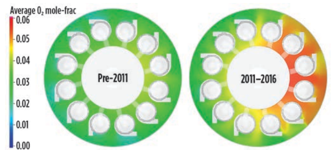
FIG. 5. Maldistribution of excess O_2 (pre-2011 and post-2011).
