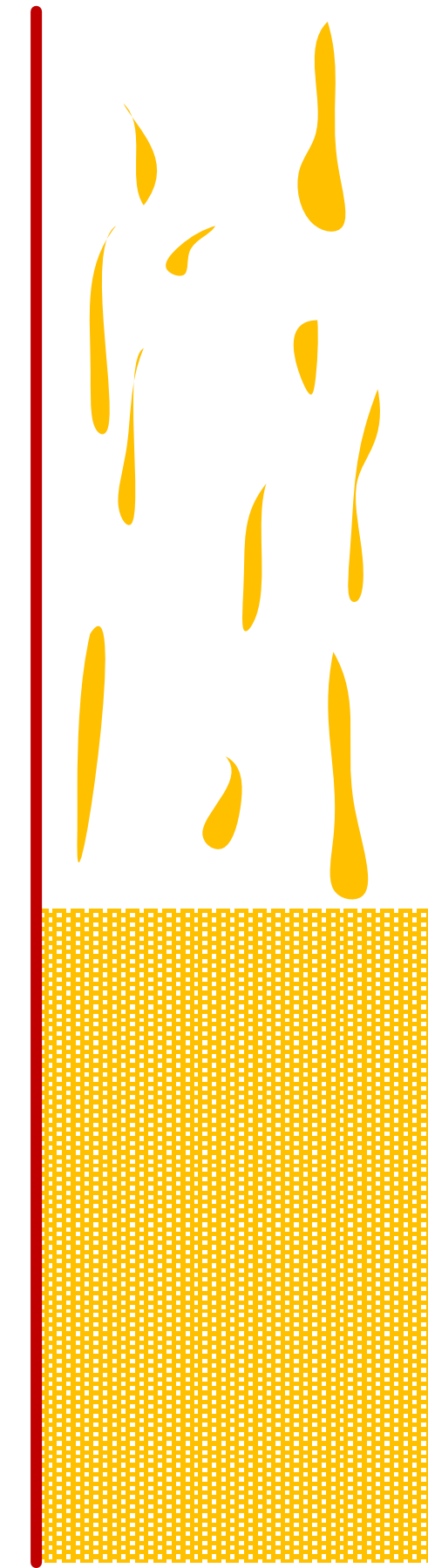
Fluid Bed with Agglomerated Particles in Freeboard
