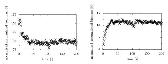
Figure 3: Normalised evolution of circulating bed material (left-hand side) and coke (righthand side) mass content within the system over simulation time in the process model
