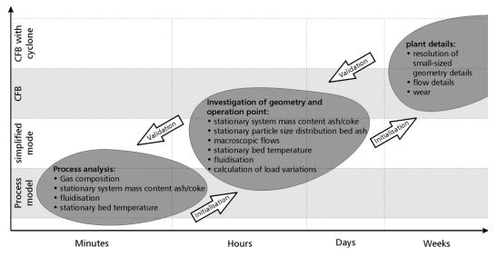
Figure 1: Flow of information with the multi-level simulation concept, Comparison of level of detail and simulation time and effort
