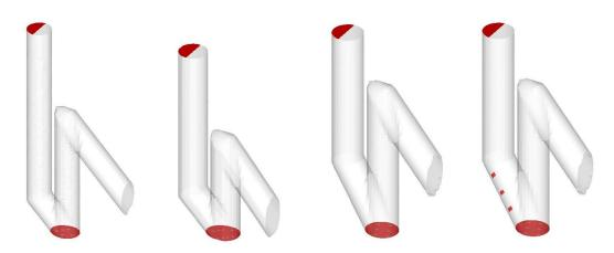
Figure 5: Evolution of basic siphon design from first design (leftmost) over a version with increased diameter (left-center), a version with increased slope angle (right-center) to version ready for detail optimisation (right).
