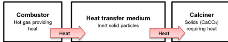
Fig. 4. Concept of indirect heat transfer from an external combustor to the calciner by means of inert solid particles
