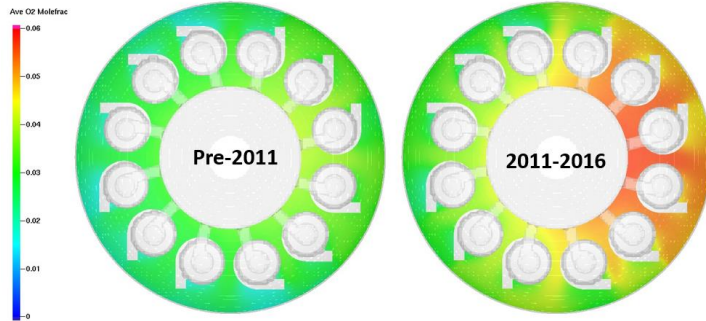
Figure 6. Maldistribution of Excess O 2
